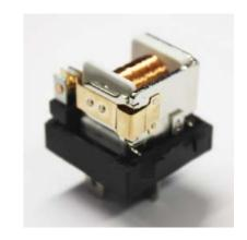
With the electronic circuits in vehicles becoming more and more fragile and sensitive, Wirez has chosen to include a Transient Voltage Protection diode in the RLY34. This diode shunts the current spike that is generated when the coil opens and prevents voltage spikes at the controlling equipment. This increases reliability and longevity of the controlling device.
